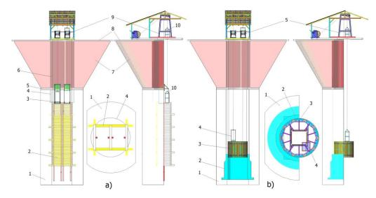
**Fig. 3.** The usage method of the equipment for the rehabilitation of the shaft by concreting, stage 1 and 2.
