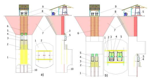
**Fig. 4.** The way of using the equipment for the Carol shaft rehabilitation, by changing the wooden armature with excavation, variant IV, stage 1 and 2.
